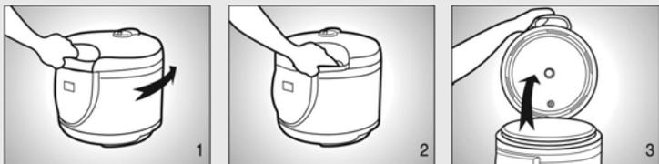
1. **How to open the lid:** When the lid (2) of the cooker is at the Closed position (Figure 1), hold the Handle (1) and turn it counter-clockwise until you reach the Opened-Lid position (Figure 2). Lift up and the lid will swing open vertically.
