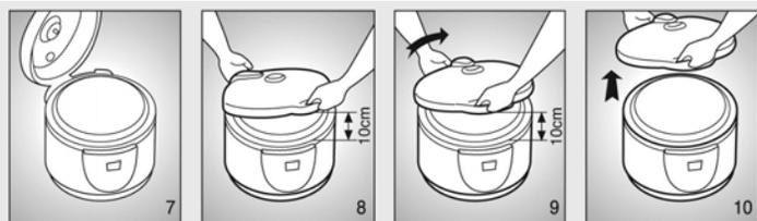
\* In the process of turning the Lid, please ensure that the height between the Lid (2) and the upper edge of the cooker is always 10cm. This is to smoothen the turning and removing process.
