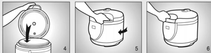
2. **How to close the lid:** When the Lid (2) of the cooker is in vertical position (Figure 4), hold the Handle (1) and close it downwards at the Opened Lid position (Figure 5). Turn clockwise until you reach the Closed Lid position. (Figure 6).
